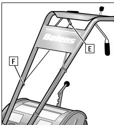
Figure 5-11: Location of forward clutch cable spring (E) and forward cable adjuster (F).
